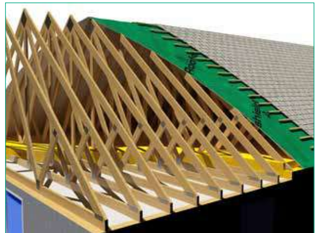
Cold Roof Construction
