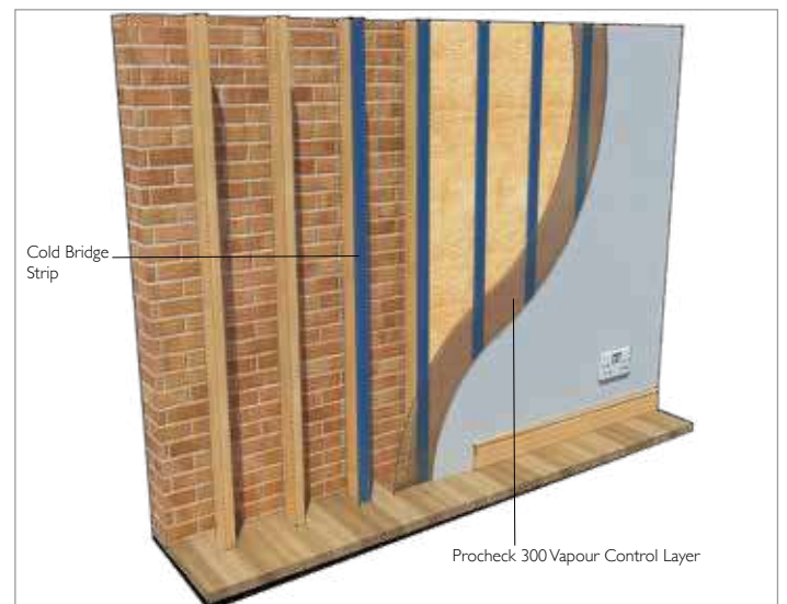
Image showing Spacetherm CBS applied to a timber frame structure
