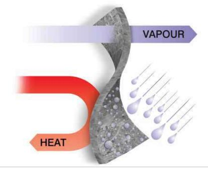
Spacetherm: Class leading thermal performance with breathability and water resistance
