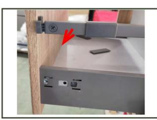
2. Pull forward the support arm to loosen the support from the drawer. Locate and remove the dark grey cover caps from the side of the drawer.
