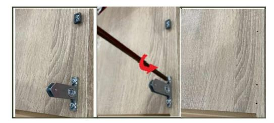
**4.** Place the released drawer on the ground with the drawer clips facing up. Insert screwdriver and twist Anti-Cloackwise to release tension and remove.
