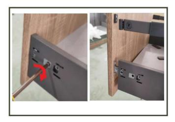
3. Using a posidrive screwdriver, insert screwdriver into the area shown above and twist 90° away from the drawer panel. This will now release the drawer panel.
