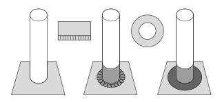
Cut flashing strips at regular intervals of approx. 30 mm and guide them around the pipe.
