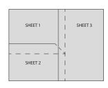
The second membrane must be given a corner cut.
