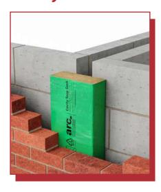
ARC's Party Wall Cavity Stop Sock is designed for use at the party wall junction; fitted in the external wall cavity, with a minimum 50mm overlap either side of the party wall cavity. At 250mm wide, ARC's PWCSS range is suitable for use with party wall cavities up to 150mm wide.
