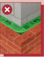
All corners and joints are tightly butt jointed. Barriers are not bent around corners.
