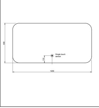
**Dimensions** (measurements in mm)
