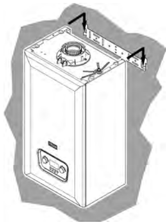
Fig.30 Mounting the boiler
