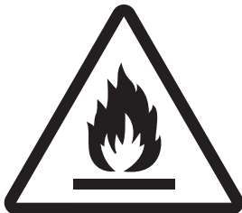
Caution: Risk of fire/flammable materials
