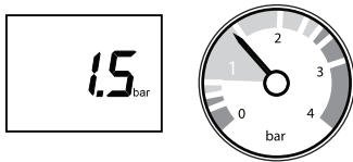
Fig.52 Restore water pressure
