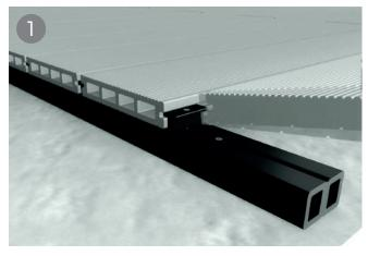
Step 1, after the last board of the main project has been laid, screw in a T clip along the edge of the final board. The bullnose board can then be inserted next to it.
