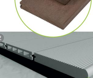
Step 2, once the bullnose board is placed you will need to insert a screw at an angle through the supporting joist underneath the board. Ensure the bullnose board is supported along the length with joists and a screw is inserted into each one.
