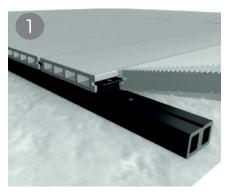
After the last board of the main project has been laid, screw in a T clip along the edge of the final board. The bullnose board can then be inserted next to it.
