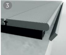
Once the bullnose board has been secured into place you can use a skirting board to neaten the edge. For higher areas you may wish to use a decking board as an edge. Secure the skirting edge with either a screw into each joist or using sumo grip adhesive.
