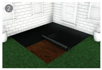
Remove the turf until the ground is completely even. Cover the area of your site with a layer of weed control fabric to prevent any weed regrowth coming up under your decking. You may want to pin your weed mat down at this stage.
