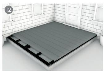
Having fastened your boards all that remains is to tidy up the sides of your new deck with our WPC skirting and corner trims which can be used to hide the unfinished end of boards and supporting joists.
