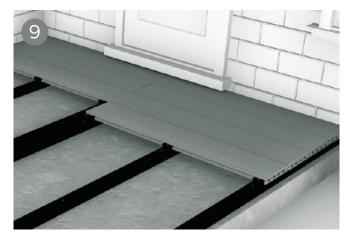
Fit your next board by sliding it onto the T-Clips used to secure the first board and fitting another set of T-Clips to secure the opposite side of the board, again one T-Clip for each supporting joist. Follow a similar process to fix subsequent boards.
