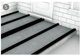
A starter clip needs to be fixed to the end of the WPC joists before laying the first board. Place these at the end of each joist where you will start to lay your boards, leaving a gap of 15mm between the wall and the end of the joist to allow for expansion.
