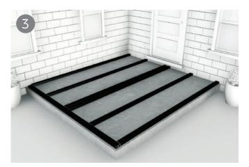
Boards must not be laid directly on the ground but should be fixed to the joists of a suitable supporting substructure. This will vary, for a domestic patio deck we typically recommend a simple concrete base and our own WPC joists.
