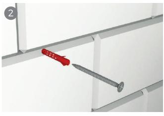
You will need to pre-drill the battens and the surface below using a 6mm drill bit, the battens are 30mm high and you will need to secure them at least 50mm into the surface below. You will need to choose fixings suitable for the surface you are fixing into. Screws should be 5-6mm diameter and at least 80mm long\*.
