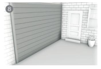
Depending on your installation, you may want to finish off the edges using one of the trims Cladco can provide to give you a lasting professional look. There are a range of trims available in all colours to compliment your cladding boards and these can be secured to your installation by glue them in place using an exterior grade high elastic glue.
