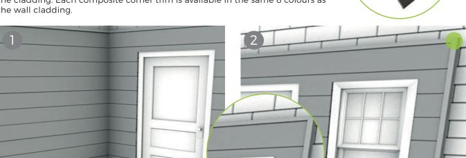
Installing the corner trims is the last phase of the project, install the composite wall cladding as above right up to any windows or doors.
