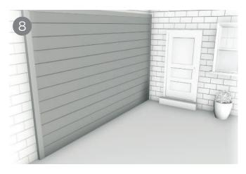
Depending on your installation, you may want to finish off the edges using one of the trims Cladco can provide to give you a lasting professional look. There are a range of trims available in all colours to compliment your cladding boards and these can be secured to your installation by glue them in place using an exterior grade high elastic glue.
