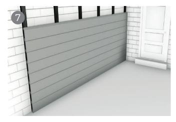
Continuing to fit the cladding boards in this manner until you have completely covered the area you want. It is possible to fit your boards side by side simply but the two ends up together. You may need to install more battens if you wish to do this as each board will need to be supported on a joist where it meets the next board.
