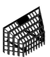
Function They are designed to stop any object that may block the efficient draining of rain water
