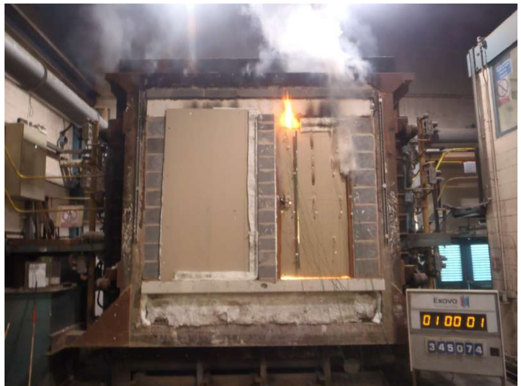
The unexposed face of the doorsets after 60 minutes of testing after which time the test was discontinued
