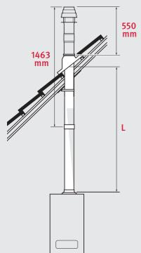
L = Flue length, measured from the top of the boiler to the underside of the roof flashing.
