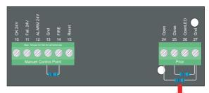
2 Connection of the Fireman's Priority Switch is made as shown on the drawing
