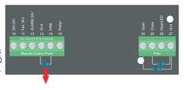
Connection of the break-glass point is made as shown on the drawing
