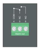
Potential free ALARM switch. COM + NO connected on alarm. Max. (30Vdc 5A) / (250Vac 5A)
