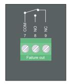
Potential free FAILURE switch. COM + NO connected on failure. Max. (30Vdc 5A) / (250Vac 5A)
