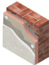
External insulation for masonry walls
