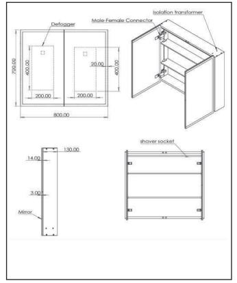
Dimensions (measurements in mm)
