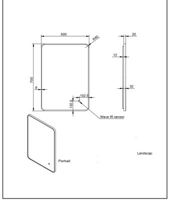
Dimensions (measurements in mm)
