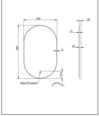
Dimensions (measurements in mm)
