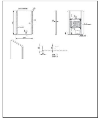
Dimensions (measurements in mm)
