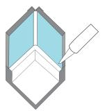
Multipanel® Seal is an all-in-one kit for sealing the bottom edge of Multipanel® at a shower tray or bath. See separate installation guide.
