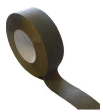
Novia Breather Membrane Lap Tape is a sealing and bonding tape suitable for sealing laps on Novia Breather Membranes within both roof and wall applications. It should be used in conjunction with Novia Double-Sided Adhesive Lap Tape for a fully sealed and airtight membrane installation.
