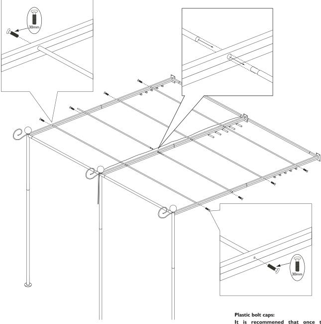
It is recommened that once the whole structure is built and all fixings have been checked to then fit the plastic bolt caps over the heads of each bolt
