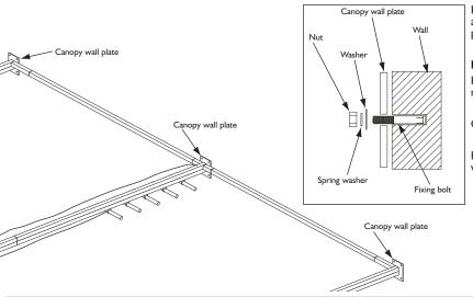
Put the canopy frame into position, ensure the feet are flat on the floor and the tracks are level using a sprit level. Mark the wall with the position of the 4 holes of each wall plate.
