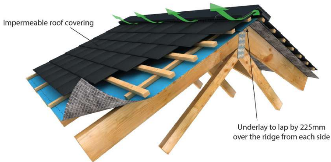
Figure 4 - Cold Roof detail with impermeable roof covering - Ridge Detail
