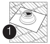
Trim the rubber boot to suit pipe size. Ensure surface is clean and dry before application.
