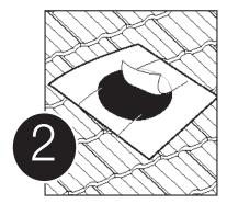
Remove the middle underside backing strip and slide the flashing
