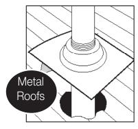
For metal roofs, remove the top backing strip and press down
