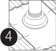
Remove the bottom backing strip and dress the base down firmly,
