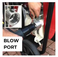
**BLOW PORT:** EXHAUST OUTLET ON HONDA MOTOR:
