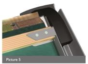
5) When tiling, all perimeter tiles must be twice mechanically fixed. Perimeter clips must be installed on each verge tile by nailing the clip through the tile nailhole when fixing the tile below (Picture 6).
