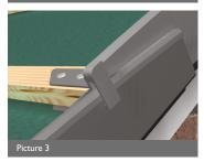
3) Fix a continuation unit to the second tiling batten and locate the clip over the top edge of the previously fixed unit (Picture 3). Nail to the tiling batten using 2 x 20mm nails. Repeat this on each course as necessary (Picture 4).
