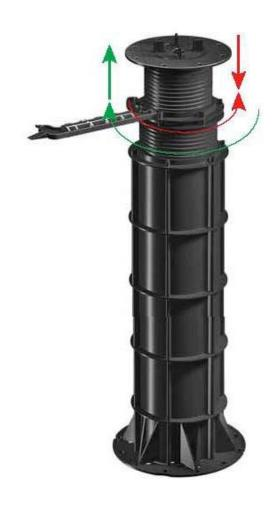
The telescopic stem (14) adjusts the height of the Megapad Pedestal finely to the millimetre. Rotate the stem clockwise to increase the height of the Megapad. The stem of both of the central column (14) and the headpiece (12) can be twisted to increase the height.
