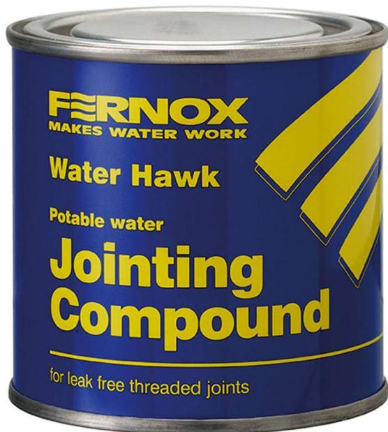
Water Hawk is a pipe jointing compound designed for use with hot and cold potable water. It is suitable for potable water, Natural Gas, steam, air (excluding medical lines) brine, alcohol and L.P. Gas. It is ideal for use on pipe diameters up to 25mm and with reinforcement fibre on pipework over 25mm. The non-toxic formulation is also WRAS approved.
