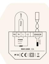
Caution: Ensure power is disconnected when wiring!
