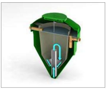
2: The draft tube enables the solids to be drawn back up into the central aeration chamber and recirculated through the treatment process.
