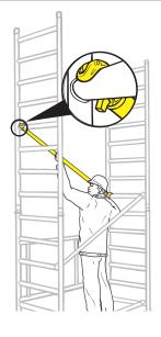
**9** Attach one stabiliser to each corner of the tower. Loosen clamp and place around vertical tube, tighten using handle. Refer to Stabiliser Section for positioning diagrams. To attach one stabiliser to each corner of the tower loosen clamp and place around vertical tube, tighten using handle.
