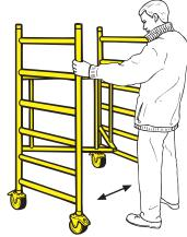
2 Push folding frame outwards until folding elbow joints lock into position. Fully unfold base frame. Ensure both folding elbow joints are in locked position (see insert). To unlock joint press latch inwards.
