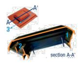
1 barrier prevents water ingress 2 barriers block wind driven rain 3 water drains away down slope
