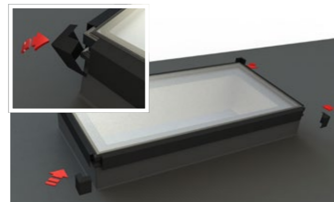
5 Fit the corner trims by hooking them under the external claddings and rotating them over, clipping them into place.
