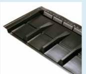
The rafter tray maintains a clear air space of either 10 or 25mm from the eaves to the roof void, by creating a barrier for the roof space insulation. Available to match all common rafter spacings.
