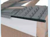
Discreet eaves ventilation which is highly effective despite being virtually invisible and is suitable for use on buildings with or without soffit overhangs and with corbelled eaves. Made from lightweight yet, very strong polypropylene, it features a 4mm grill stopping large insects or small rodents getting into the roof void
