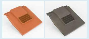
A neat and compact design that will maintain the aesthetics of a plain tile roof. This vent is designed for use with the standard 265mm x 165mm plain tile, replacing only 3 tiles without the need to cut any roof battens or surrounding tiles.
