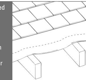
If Vent3® underlays are to be installed over a fully supported system you must install 12mm counter battens over the underlay, using corrosion resistant clout nails. Ensure there is an uninterrupted space between the underlay & roof tiles or slates to provide adequate drainage.
