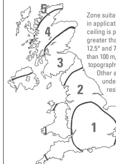
Zone suitability applies only for underlays in applications where a well-sealed ceiling is present, ridge height is not greater than 15 m, roof pitch is between 12.5° and 75°, site altitude is not greater than 100 m, and no significant site topography is present.
