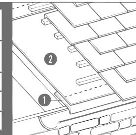
1. Use support tray or protection strip to extend into the gutter, then overlap with a first run of Vent3® colour side uppermost, eaves, and work up the slope of the roof.
