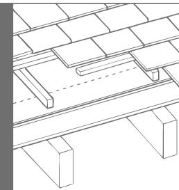
For unsupported applications drape the underlay by a minimum of 10mm between the rafters to allow the water to run off.
