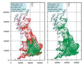
Ridge height 11.0m Mid altitude Roof pitch 30° Underlay rating 1.0kPa Ridge height 11.0m Mid altitude Roof pitch 30° Underlay rating 2.5kPa
