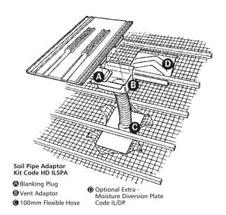
Fitted flush with the slates at 2 m centres, the ventilator will provide an equivalent airflow to a continuous 5 mm high level gap, and should be fitted in conjunction with the appropriate Hambleside Danelaw eaves ventilation products. As an alternative to an eaves ventilation system the vents should be fitted at 1 m centres to achieve the equivalent of the requirement for a 10 mm continuous gap at eaves
