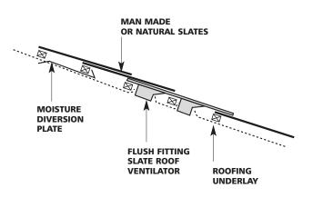
Flush Fitting Ventilator to suit two slate sizes:-600mm x 300mm Code HD ILSRV10/24 500mm x 250mm Code HD ILSRV10/20
