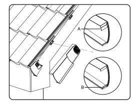
5. Next, clip the first verge unit onto the starter unit; this will require the flange tab A (code HD IDV) or B (code HD TIDV) on the first verge unit to be snapped off at the break line. Once firmly clipped to the starter unit, the verge unit can then be nailed through one of the holes provided into the batten end or continuous batten. Where the batten end clip is used, the nail should penetrate one of the slots provided.
