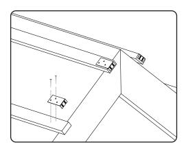
2. It is recommended that batten end clips (code HD IDV/BC) be used at the batten ends to provide long term secure fixing. One clip should be nailed twice to the top of each batten with the short flange in contact with the batten end.
