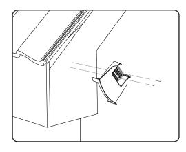
4. The verge starter unit (code HD IDV/ST) should be fixed securely at the eaves through the slots using the 2 x 25mm flange head screws provided into the barge board or masonry. The starter unit is most easily marked for position by fitting to a verge unit and placing the verge unit onto the eaves tile.
