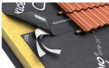
Permo® forte SK<sup>2</sup> has a double integral tape at the laps. This creates a very effective and secure airtight seal, reducing energy loss.
