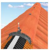
Place end ridge tile centrally over the white spine of the Roll-Fix® and insert ridge seal under and between ridge tiles. Secure using the 100mm screw, washer and clamping plate provided. Continue this process along the ridgeline to the abutment, hip
