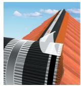
Starting at one cite, in the Roll-Fix® centrally over Starting at one end, unroll the ridge batten, making sure there is 75mm cover each side of the top course of tiles. Secure in place using corrosion resistant nails or staples at 300mm centres through the white spine of the Roll-Fix®.
