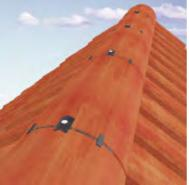
Place end ridge tile centrally over the white spine of the Roll-Fix<sup>®</sup> and insert ridge seal under and between ridge tiles. Secure using the 100mm screw, washer and clamping plate provided. Continue this process along the ridgeline to the abutment, hip or gable.
