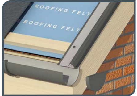
Fig.1. Nail each length of trim to batten.
