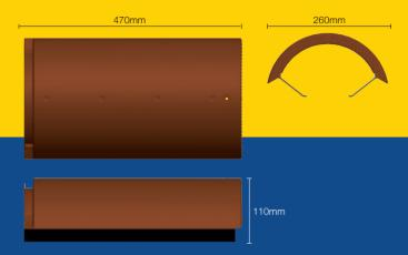
The interlocking system makes the tiles very easy to fit and, when completed, ensures an extremely secure finish.
