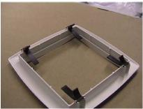
31 Remove the ducting's protective film, exposing the highly reflective mirrored surface.
