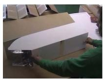
6 You can now see how the adjustable hinge works, be careful not to over bend at this stage as. Put this assembly to one side for later use.
