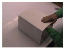
8 Cut the silver tape to the length of the joint, remove the backing tape and stick over the jigsaw joint. Smooth the tape down on the top surface and then flip the duct over and push firmly down from the inside along the jigsaw edge to make sure the edges are all in firm contact with the tape.
