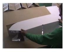
5 Flip over so that the two square touching edges are facing upwards. Tape this joint only, making sure that the two square edges are firmly pushed together as this is the hinge point. It is important to cut off the tape to the exact width.
