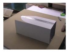
4 Now repeat the above to finish up with two identical long lengths of ducting as shown. Now slide one inside the other making sure the three cut flaps slide inside the square edges of the other and push together until the two square edges touch.
