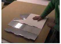
2 Bring the two jigsaw type ends together, fitting them as you would a jigsaw making sure they fit flush with each other and do not overlap.
